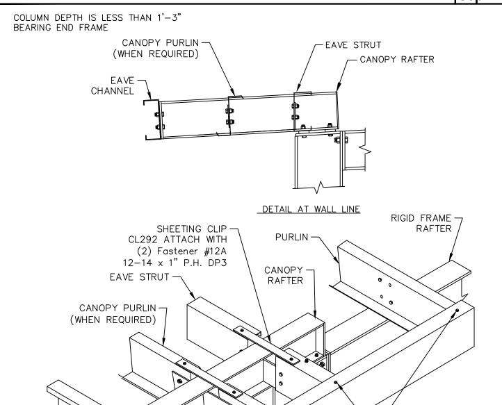
NOTES: ALL BOLTS TO BE ½"Ø UNLESS NOTED. FOR REQUIRED LENGTH REFER TO GRIP TABLE ON CUSTOM ERECTION DRAWINGS.
